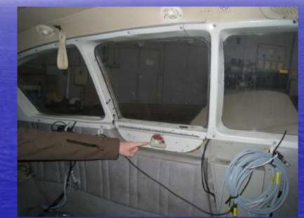
The opening of the emergency exit is done only under the pilot or experimenter order.
