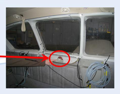
The opening of the emergency exit must only be operated under the Captain or the experimenter order.
